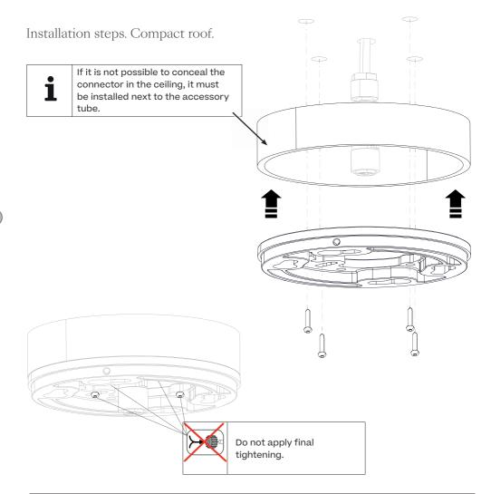
Attachment fittings are not supplied, as different roof materials require different types of fittings. The installer must ensure that these fittings can support 4 times the weight of the fan.
