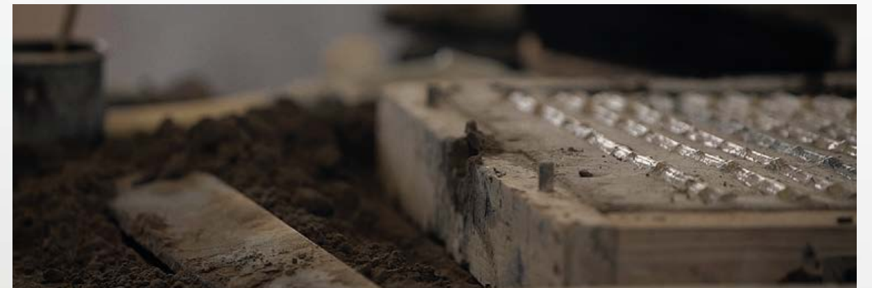
The brass casting process is made with sand, fire and brass. The melted brass fills the shapes and textures left on the sand by the branches and the leaves.
