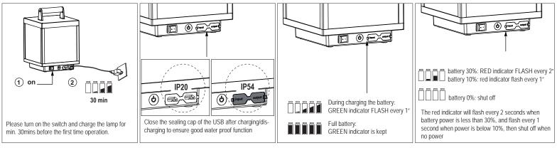
NOTE: It will dim off the lamp and no dimming when charging, also no discharging function in this situation; Never short circuit the imput and output of the lamp, or pls restart the lamp with switch.
