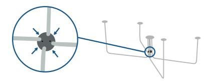
2 Fix the top fixing plate (B) to the legs with an Allen key.
