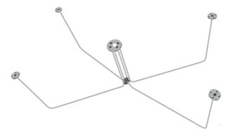
Then turn down the legs structure and place it on the table top (which must be upside down). Screw the top fixing plate (B), and then take each leg to its correct position (marked on the top) and screw it.
